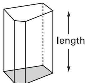
$$\text{Volume} = \text{area of cross-section} \times \text{length}$$
